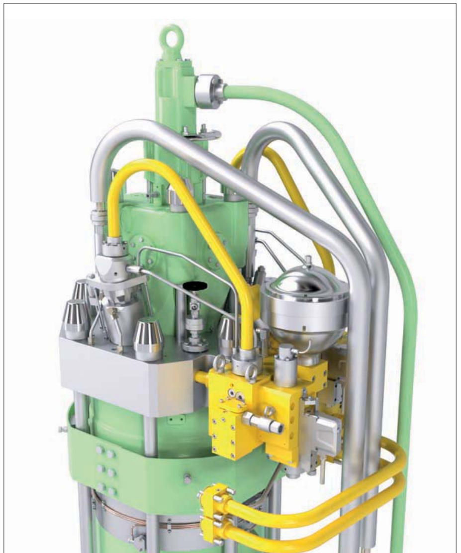
Design of the ME-LGIP cylinder cover with LPG injection valve (FBIV) and gas block Source: MAN
