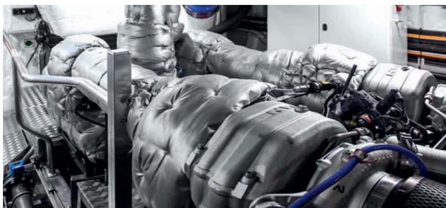
The compact and maintenance-free exhaust gas aftertreatment system from MAN Engines with selective catalytic reduction mixer, AdBlue© fluid metering unit and SCR catalytic converter (everything fully insulated). The selective catalytic reduction system enables compliance with the IMO Tier III and US Tier 4 emission standards. Source: MAN Engines/Andrew Chin
