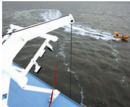
Davit system for open lifeboats Source: d-i davit
