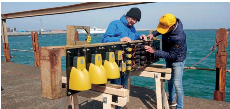
Laboratory tests are complemented by real-life tests: interim analysis after six months, during one-year outdoor testing of Extreme switchgear in maritime conditions
