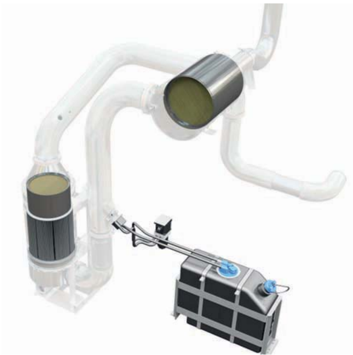
HJS project example of an autarkic SCRT-upgrade for a stationary engine Source: HJS
