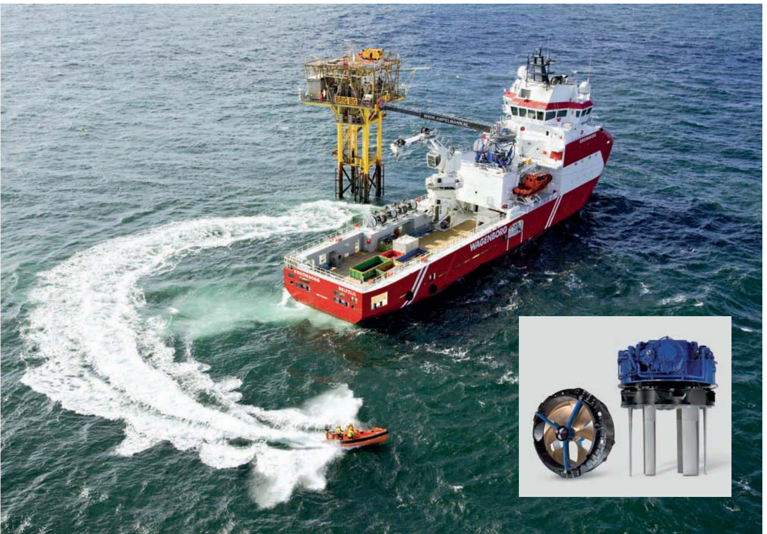
Figure 1: Walk-to-work (W2W) vessel Kroonborg : DP2; 2 x Voith Schneider Propellers and 2 x Voith Inline Thrusters; the VIT and the VSP are shown on the right Source: Voith
