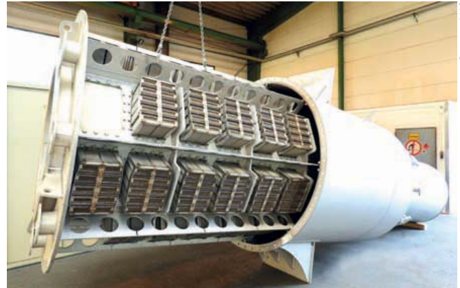
HJS - Sintered Metal Filter (SMF®) implemented in an ETB exhaust gas aftertreatment system for a high-powered marine engine
