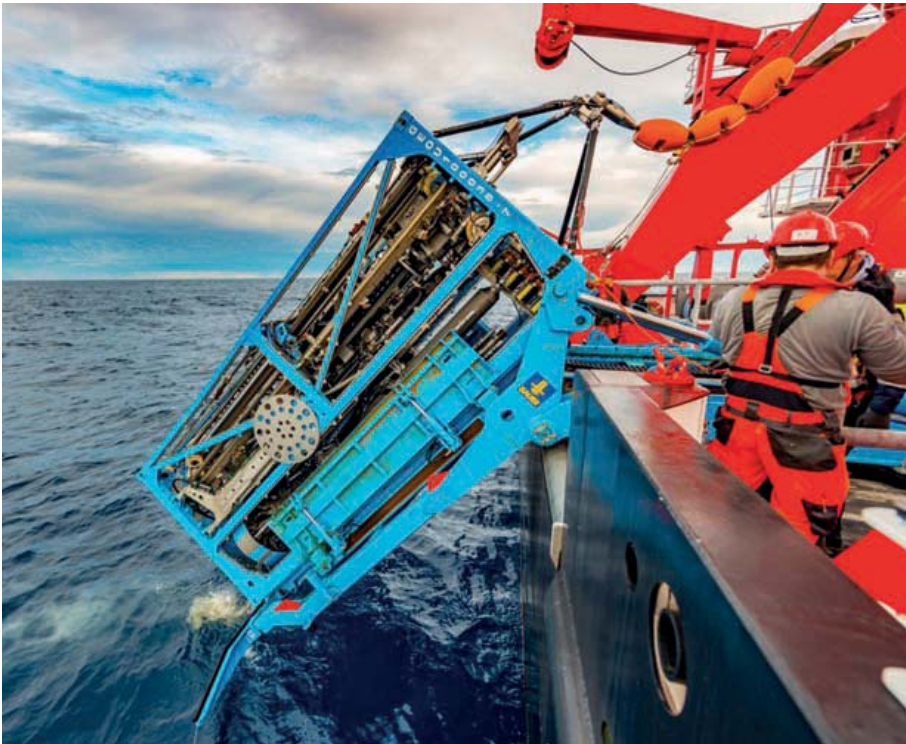
The sea floor drill MeBo can work at a water depth of up to 2,500m and can drill cores up to 200m
