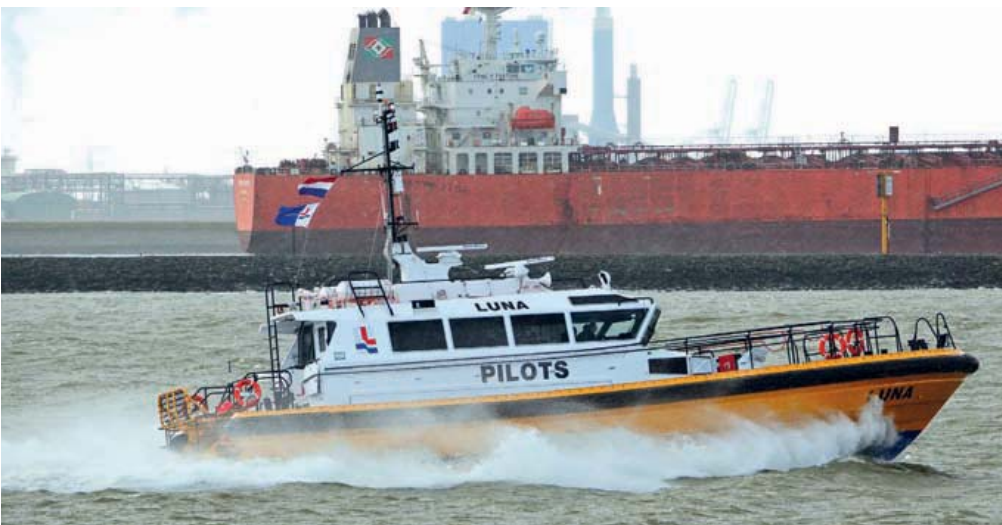
The Luna in service at the Port of Eemshaven. The pilot vessel has a three-man crew and can transport up to twelve pilots at a time. Source: Barkmeijer Shipyard
