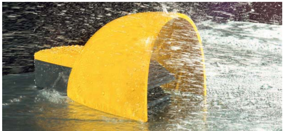
Extreme switching devices are tested in standardised laboratory conditions – e.g. for splash water protection and corrosion resistance Source: Steute Technologies GmbH & Co. KG
