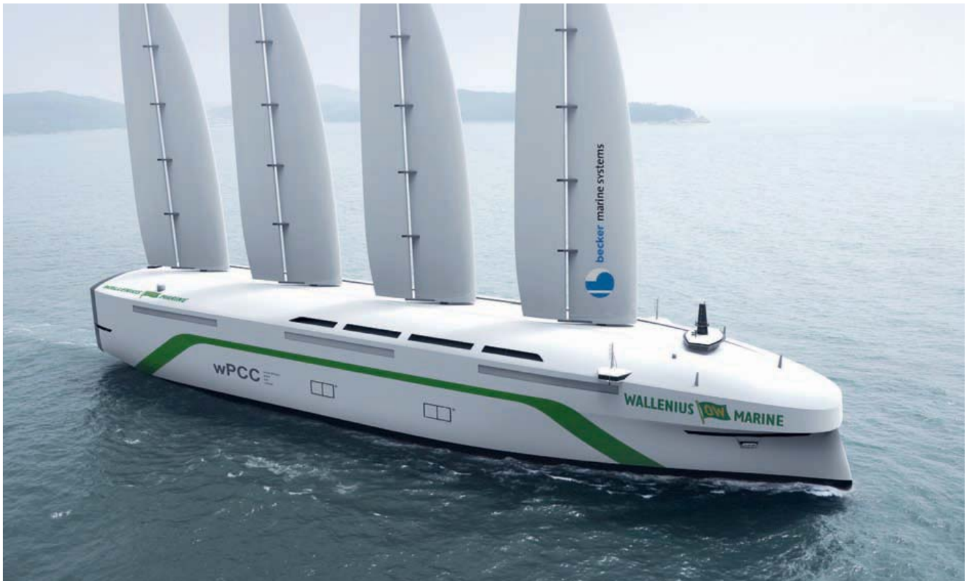
Becker claims that four wing sails will provide sufficient power to propel the vessel at speeds of up to ten knots in ideal conditions without engine support
